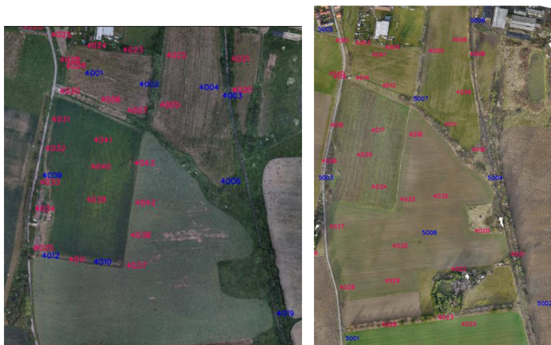
Fig. 1: Placement of input (blue) and control points (red) in the first and second measurement steps
